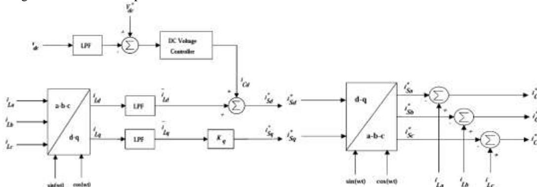
Fig. 5 Shunt compensator control scheme for generation of reference compensator currents
