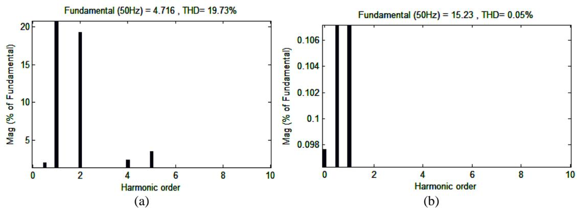
Fig.18 Spectrum of the source current in phase 1 for SRF Control (a) Without UPQC (b) With UPQC
