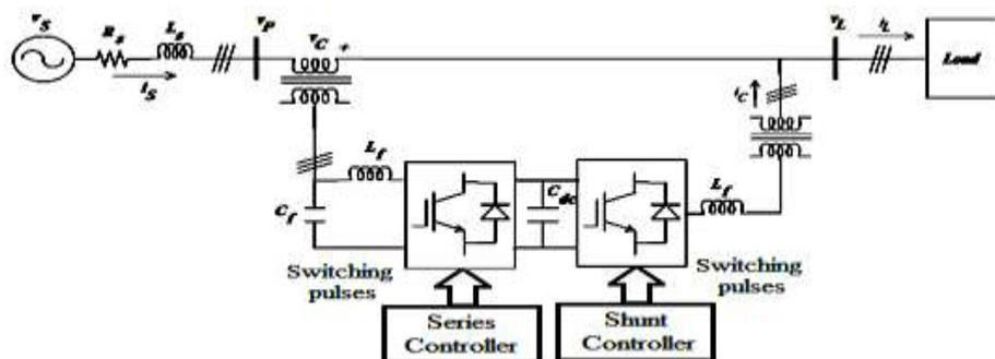
Fig.7 System Configuration of UPQC
