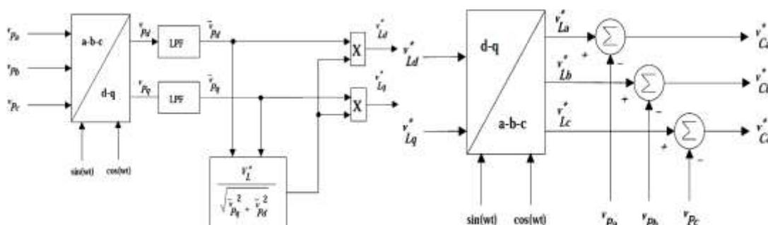
Fig.6 Series compensator control scheme for generation of reference compensator voltages
