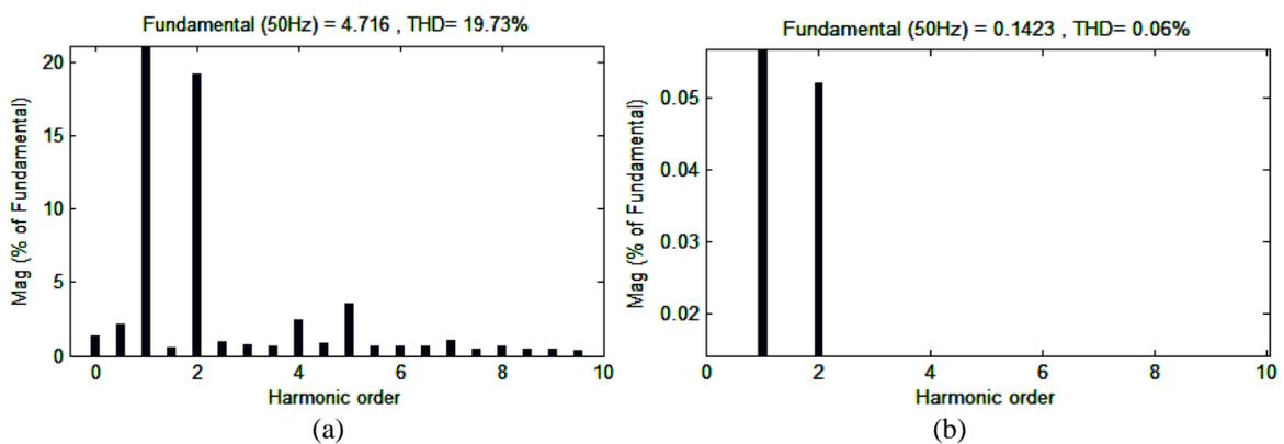
Fig. 14 Spectrum of the source current in phase 1 for PI Control (a) Without UPQC (b) With UPQC
