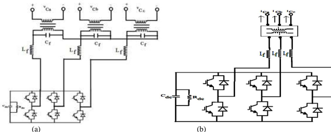
Fig. 8 Power circuit of UPQC for indirect PI control (a) Series Converter (b) Shunt Converter
