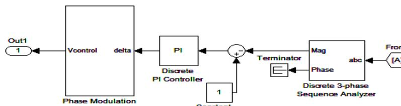
Fig. 4 Simulink model of UPQC Controller
