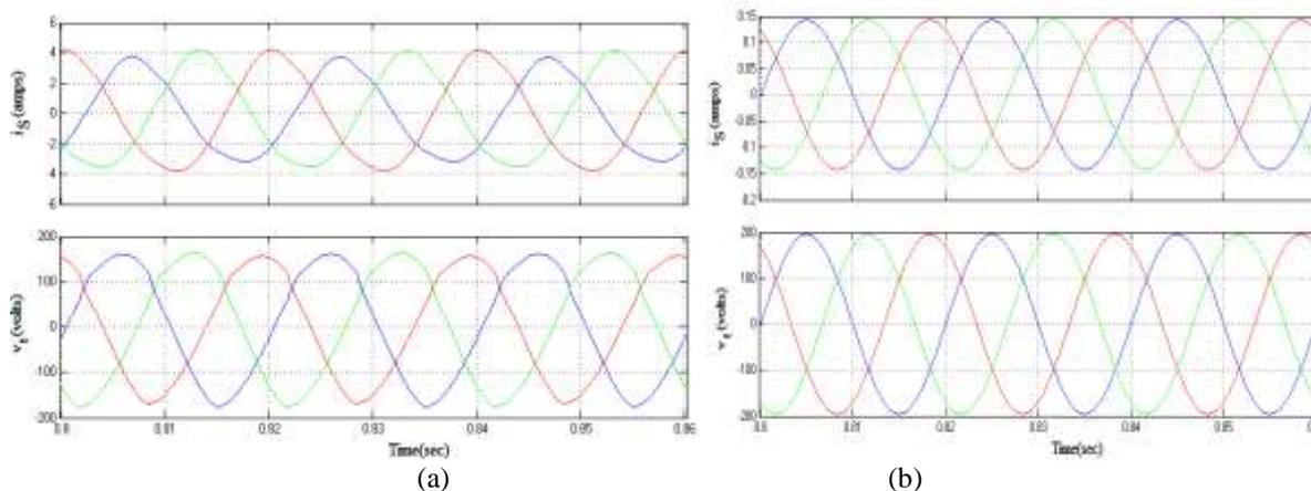
Fig. 12. Power factor correction of distribution system in PI controller (a) without UPQC (b) with UPQC
