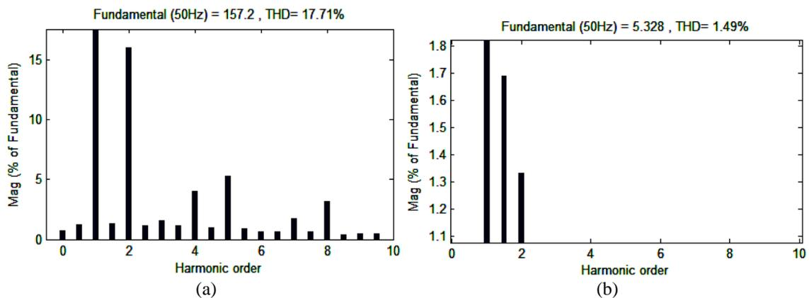
Fig.19 Spectrum of the load voltage in phase 1 for SRF Control (a) Without UPQC (b) With UPQC
