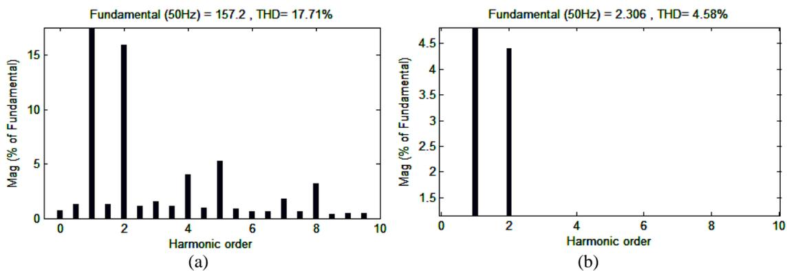
Fig. 15 Spectrum of the load voltage in phase 1 for PI Control (a) Without UPQC (b) With UPQC
