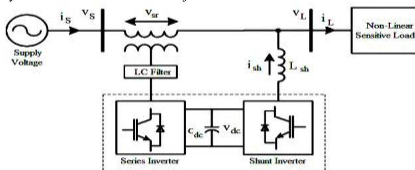
Fig 1 UPQC general block diagram representation
